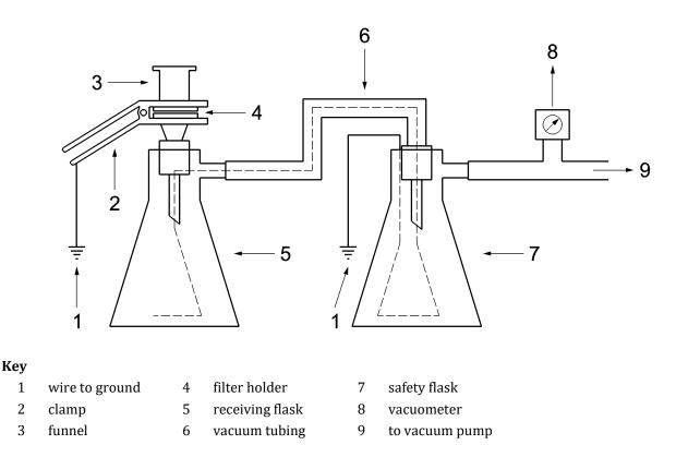
Figure 1 — Filtration apparatus for determining contamination
